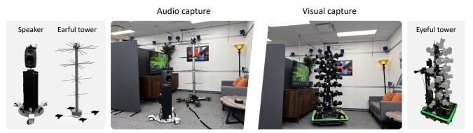
Figure 1. **Data capturing setup.** (a) Audio capture (left): the loudspeaker and microphone recording system (Earful Tower) are placed at different locations within the room to measure and capture RIRs. (b) Visual capture (right): the camera rig (Eyeful Tower) moves around rooms to capture multi-view images for visual reconstruction and novel-view synthesis.
